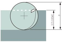
Recommended cutting width in face milling
