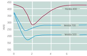
Hardness profile of gas-cut edge, cut in air
